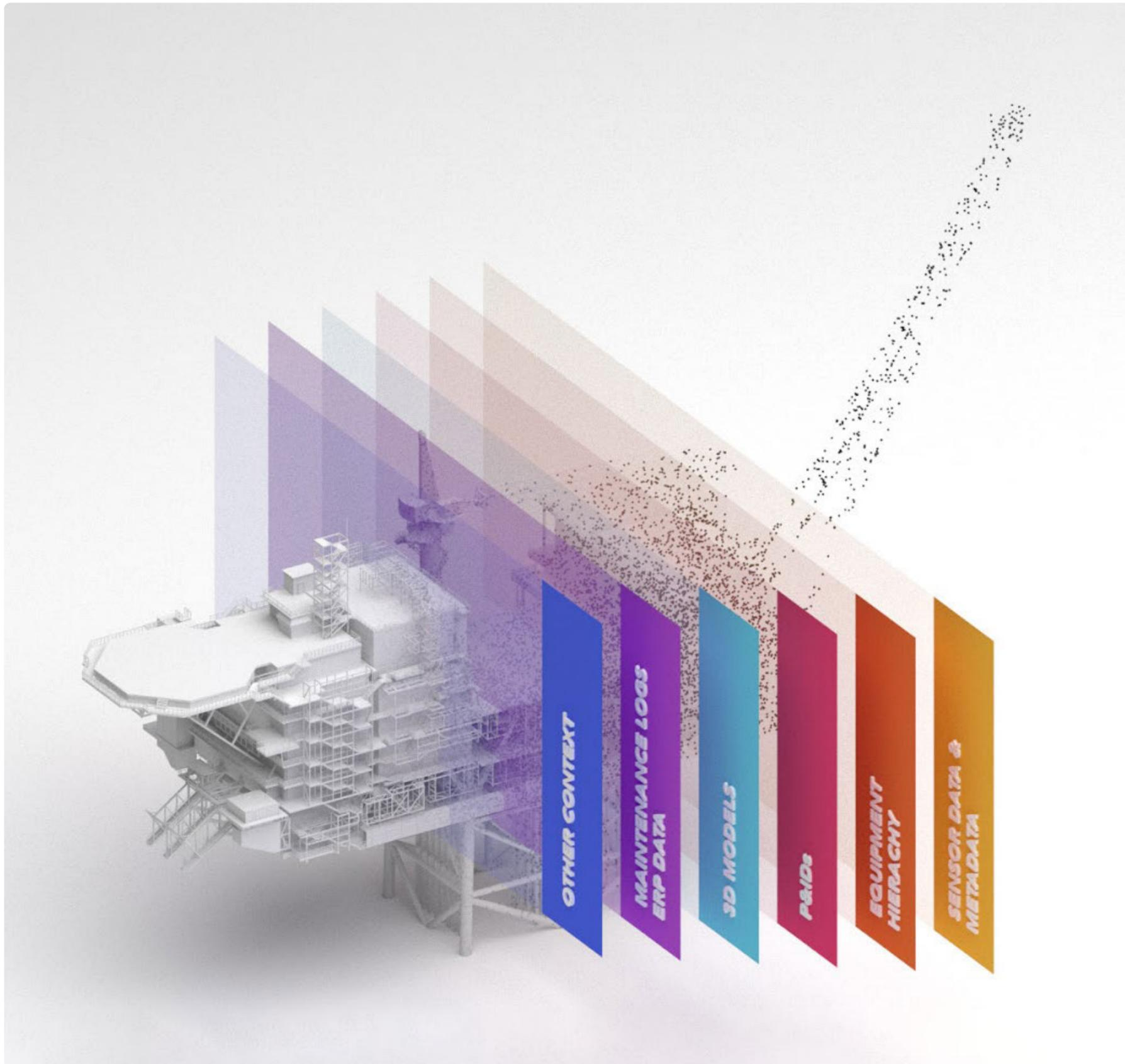
An operational digital twin is the aggregation of all possible data types and data sets, both historical and real-time, directly or indirectly related to a given physical asset or set of assets in a single, unified location. The collected data must be clean and contextualized, linked in a way that mirrors how things are or would be linked in the real world, and made consumable depending on the use case.
